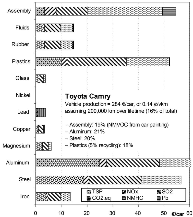
Figure 2. Contribution of materials and vehicle assembly to damage cost of vehicle production.
