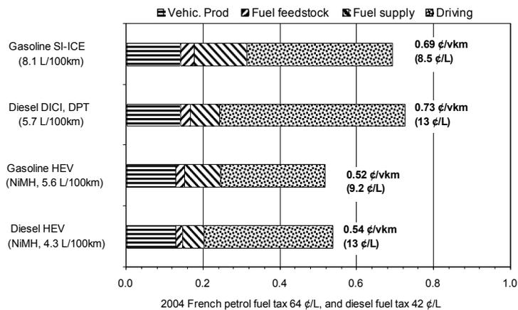
Figure 5: Damage costs of gasoline and diesel passenger cars in Europe (2010 time horizon).
