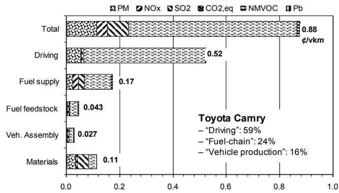
Figure 3. Contribution of the pollutants to the well-to-wheel and vehicle production stages.
