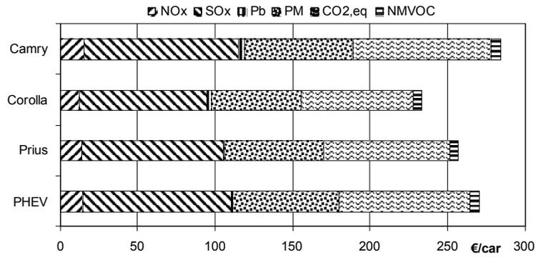
Figure 1: Damage cost due to the vehicle production stage.
